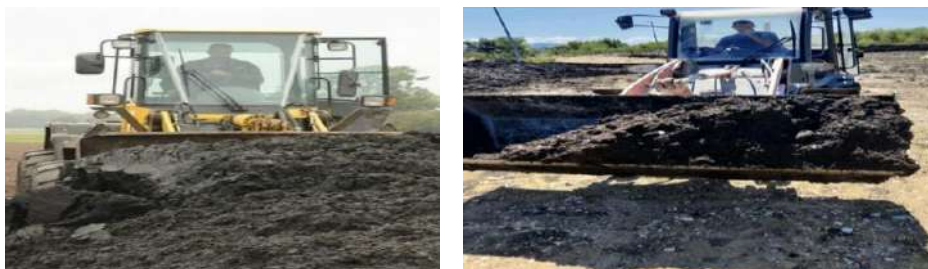
Figure 4 Outlook of, after second stage waste water treatment sludge, two years aged, with 20 % dry matter, before treatment
