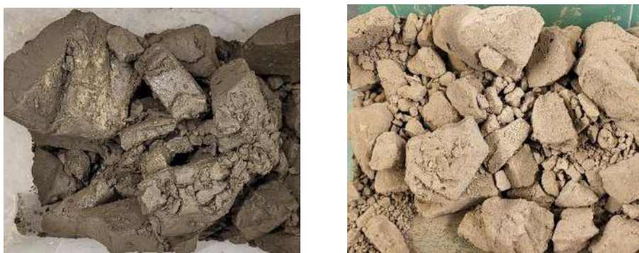
Figure 1 Fine basalt dust before and after drying
