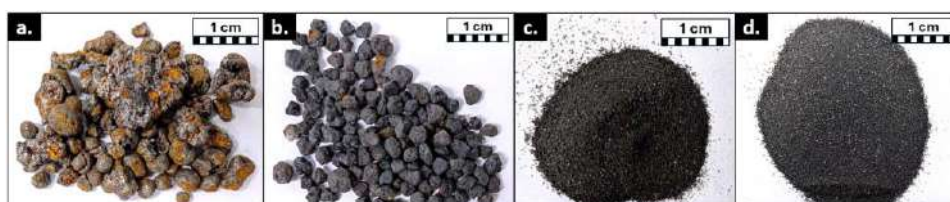
Figure 3 Grain fractions in EAFS sample FG02 after EHF processing. Liberated and hand-sorted grains from the >1 mm magnetic fraction showing the effectiveness of phase separation by EHF processing of metallic components (a.) from the slag-matrix (b.). No visual differences between the magnetic (c.) and non-magnetic fraction (d.) for smaller grain sizes (< 250 \mu\text{m} ) could be identified.
