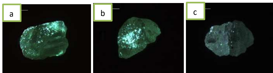
Figure 3 Fixation of luminophore-containing composition MLA-3 (E-515-115+CCHGO+DTF) on weakly luminescent (a), anomalously luminescent (b) diamonds, and a kimberlite grain (c)
