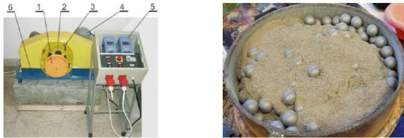
Figure 3 Laboratory vibratory mill test stand and view of the chamber interior with the ground material: 1 – chamber, 2 – chamber holder plate, 3 – drive module, 4 – vibrator motor, 5 – control and power system, 6 – supporting structure
