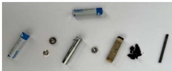
Figure 1 Zn-C batteries and their individual parts
