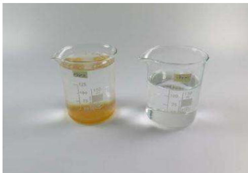
Figure 3 Retentate and permeate after titration with NaOH
