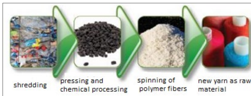
Figure 1. Textile recycling process [3]
