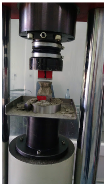
Figure 3. Testing the compressive strength of the samples
