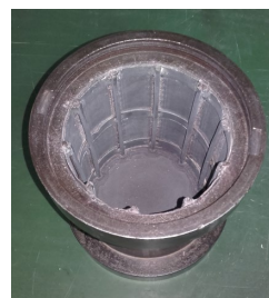
Figure 3. Ribbed inside surface of the mill
