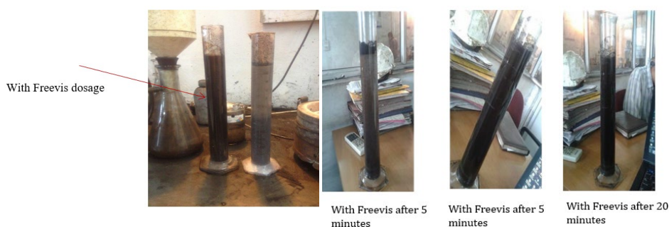
Figure 2. Comparative Test to check the effect of Freevis in magnetite suspension
