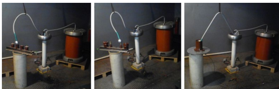
Figure 3. Measuring partial discharge of insulators
