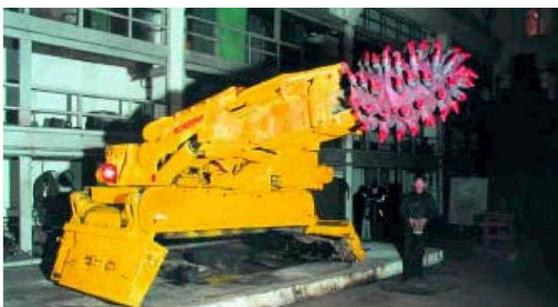
Figure 3. Remotely controlled support-walking roadheader (model KPA-3M)
