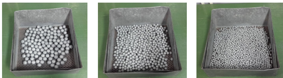
Figure 4. Three different charge made of balls of diameter 24, 15 and 10 mm
