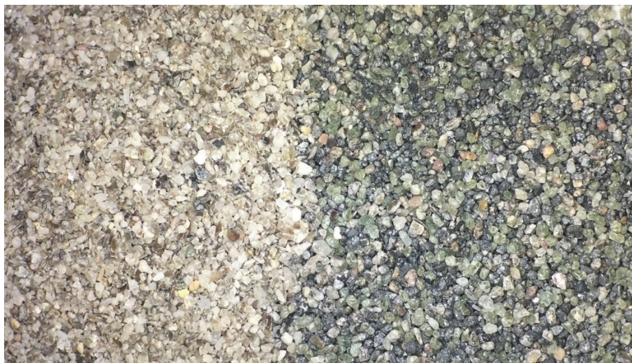
Figure 2. Photograph illustrating two final products after air gravity concentration table (light fraction on the left and heavy fraction on the right)
