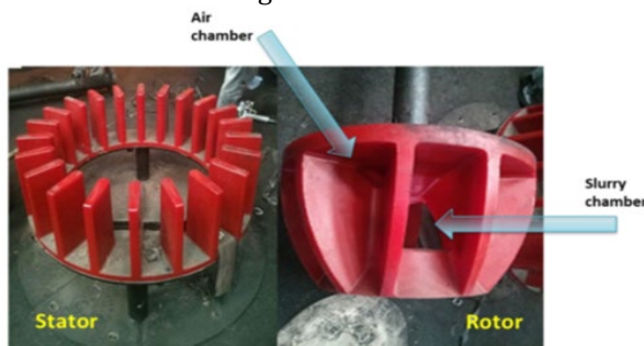
Figure 4. New generation mixing mechanism Outotec FloatForce®
